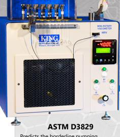
Predicts the borderline pumping temperatures (BPT) of engine oils over a 16 hour cooling cycle from 0°C to -40°C.
