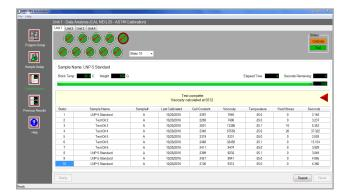
The King MRV Automation Software Package calculates yield stress, viscosity, and Rotor/Stator Cell Constants. It offers simple user prompts to facilitate the testing process and comes installed on the laptop computer.
